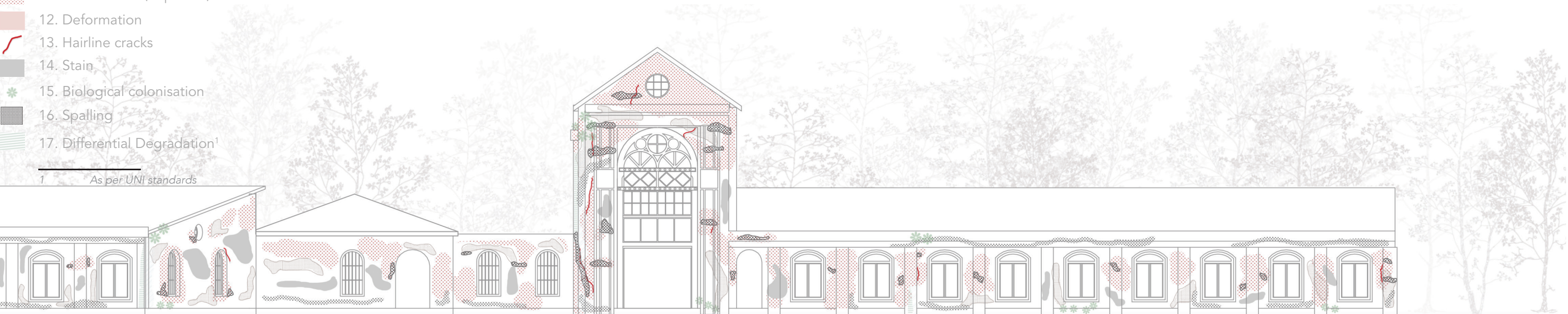
Fig. 279 Decays on the North elevation of the area in focus © Author
