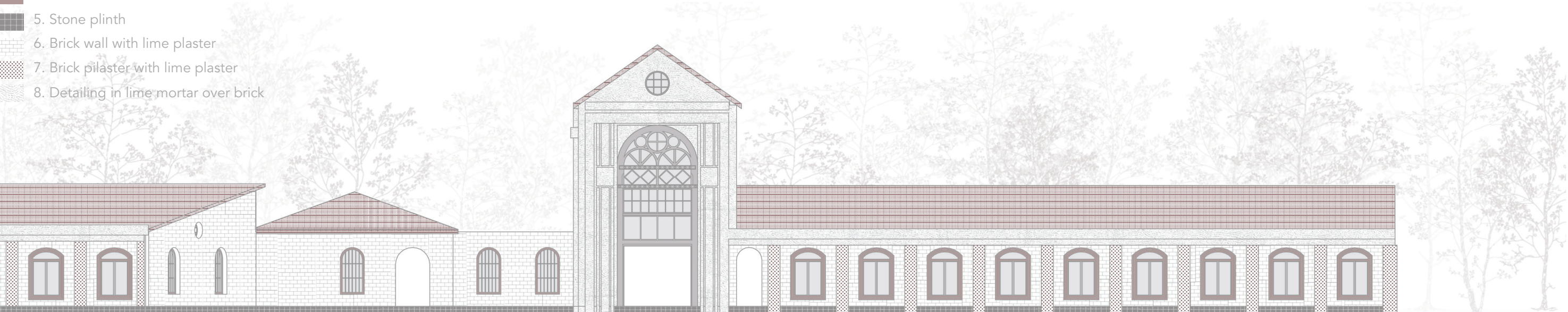
Fig. 279 Building materials in the North elevation of the area in focus © Author
