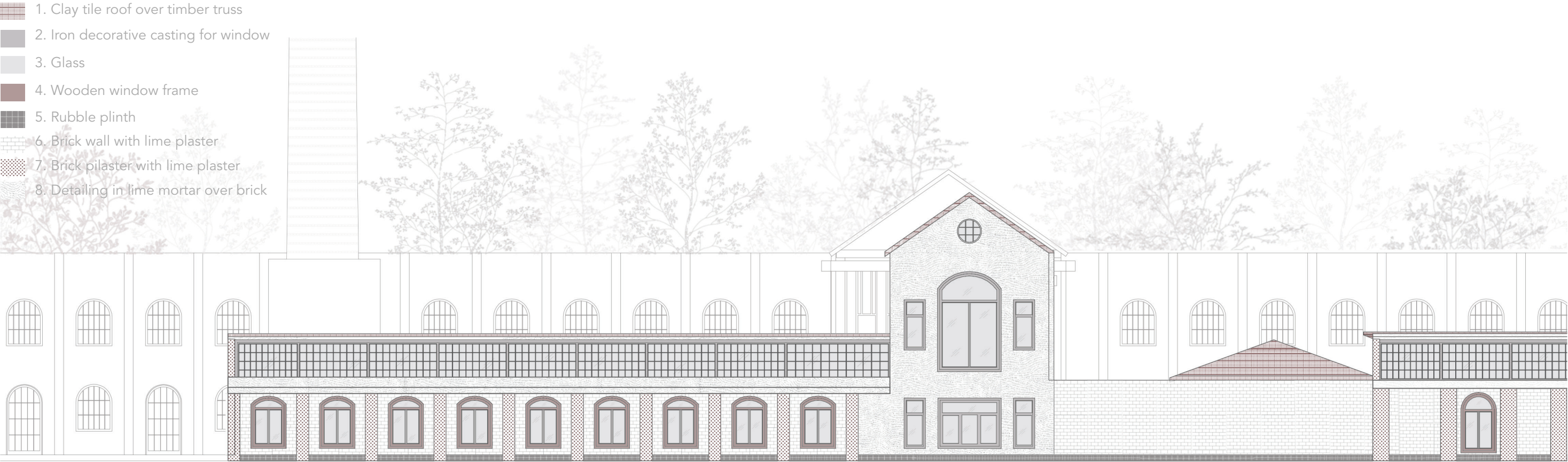
Building materials in the South elevation of the area in focus © Author
