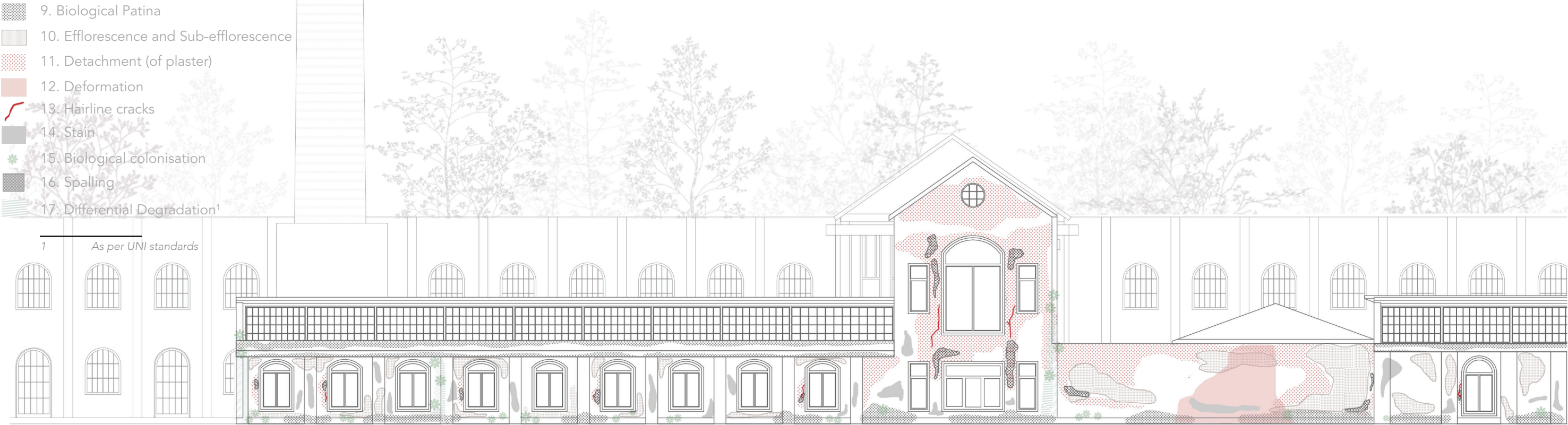
Decays on the South elevation of the area in focus © Author
